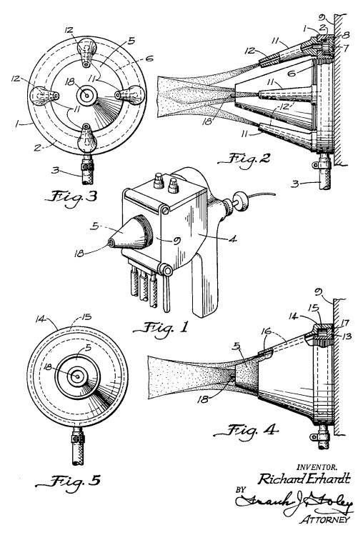
nozzle a number of jets such as 11, each having a duct 12 may be secured in any suitable manner, for example, as shown, to the manifold for conducting the hydrogen gas forwardly toward the end of the nozzle. I have found that four jets are adequate for the
